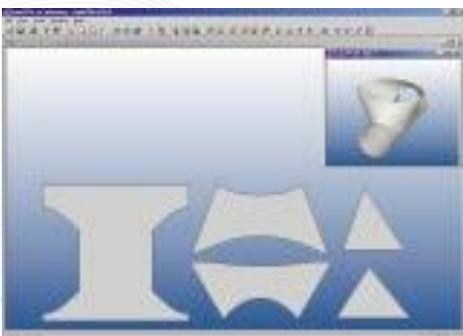
Configurable output when exporting unfolded geometry's as DXF files. Line types and colours can be selected. Bend angles can be included.
